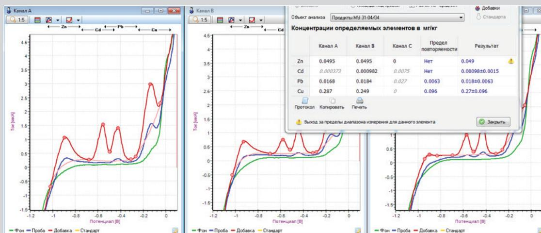
Figure 1: Voltamperogram of the content of mass concentrations of Zn, Cd, Pb, Cu in canned cucumbers.
